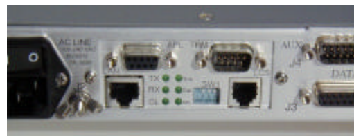
SMR5000HL Rear Panel Interface Connections
